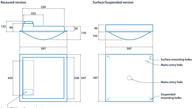
3-pole TEE (SmartScan versions) Fast-Fix wiring enclosure (Non-dimming and DALI versions)
